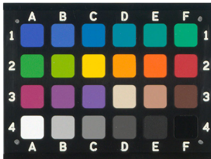
Figure 2. sRGB image of the Artist Paint Target. Image Science Associates manufactured the sample holder.
