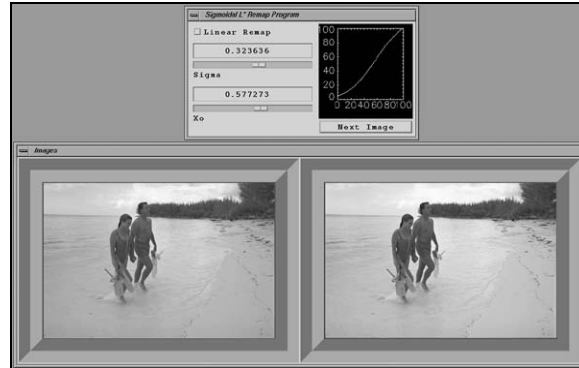
Figure 5. User interface for adjustment experiment. The subjects adjusted the x_0 and \sigma sliders until the reduced dynamic range image (right image) was the best possible match to the original full dynamic range image (left image).
